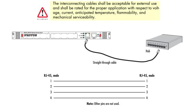
Figure 14. Typical Ethernet straight-through cable diagram for 10/100Base-T
